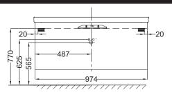
Product Specification: BASE unit 97.5 cm. EB1047. Collection: REPLAY. Dimensions: 97.5 x 45 x 47. Weight: 40.1 kg. Installation: Wall-hung with or without feet.
