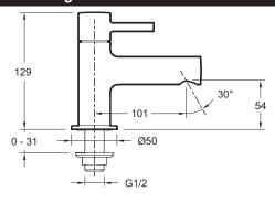
Product Specification: Pillar tap for handwash basin. 37308D. Collection: CÜFF. Weight: 1 kg. Installation: 1 hole. Normes: ACS (Certificate of Sanitary Compliance):10 ACC LY 239. Flow rate: 5 l/mn. Flow rate: 5 l/mn. Height under spout: 129 mm. Connection: With supply hoses. Mechanism: Quarter-turn ceramic disc cartridge. Rotating anti-scale aerator. Waste. Finger imprint on handle for better grip. Height under aerator: 54 mm.
