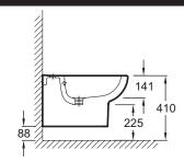
Product Specification: Wall-hung bidet 54 x 36.5 cm. 4953K. Collection: REACH. Dimensions: 54 x 36.5. Weight: 19 kg. Material: Ceramic. Installation: Wall-hung. Wall-hung. easy floor cleaning. Standard fixings: easy installation on support frame. Chromed overflow cap.
