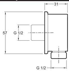
Product Specification: Wall elbow, round. E75142. Collection: NO COLLECTION. Weight: 0.4 kg. Incl. non-return valve.
