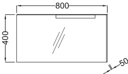
Product Specification: Mirror 80 cm. EB2007. Collection: STILLNESS. Dimensions: 80 x 5 x 40 cm. Weight: 21 kg. Installation: Wall-mount. Power : 230 V, 8 W, class II IP44, energy efficiency class A++-. Anti-steam feature. LED light at top & bottom. Lighting: 230 V, 8 W, class II, IP44, energy efficiency class A++-.
