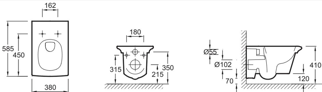
Product Specification: Wall-hung WC pan 58.5 x 38 cm. 2537W. Collection: STILLNESS. Dimensions: 58.5 x 38. Weight: 25.6 kg. Material: Ceramic. Installation: Wall-hung. Fixings: Concealed fixings included and metal band in option. Hole configuration: Fixing centre: 180 mm.. Unique design with fluid, dynamic lines. Smooth-sided, no dirt traps, for easier cleaning. Slow-close thermoset seat, metal hinges, E6369.. Water saving 3/6 L dual flush. Can fit into cabinet.
