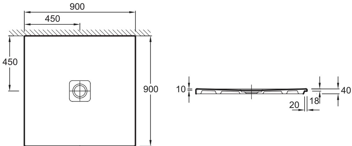
Product Specification: Extra-slim square ceramic shower tray 90 x 90 x 4 cm. N140K. Collection: REPLAY. Dimensions: 90 x 90 x 4. Weight: 31 kg. Material: Ceramic. Installation: Floor-standing or inset. Shape: Square. Shape: Square. Floorstanding or inset. Anti-slip glaze. Order with special drain and cover 9276K. Waste Ø 90 mm.
