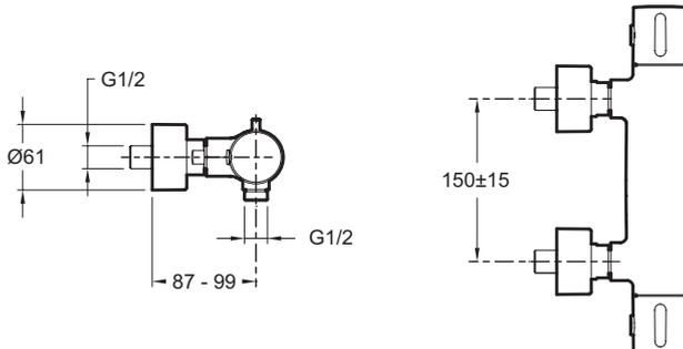
Product Specification: Thermostatic single-lever wall-mount shower mixer. 37035D. Collection: CÜFF. Weight: 3.1 kg. Installation: Wall-mount. Normes: ACS (Certificate of Sanitary Compliance): 10 ACC LY 102. Connection: With connectors and wall escutcheons. Mechanism: Expandable wax cartridge. Hole configuration: 150 ± 15 mm. On temperature handle: Safety stop at 38°. Maximum temperature limited to 50°. Integral anti-scale aerator. 5-year guarantee.
