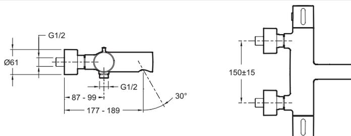
Product Specification: Thermostatic single-lever wall-mount bath/shower mixer. 37037D. Collection: CÜFF. Weight: 3.6 kg. Installation: Wall-mount. Normes: ACS (Certificate of Sanitary Compliance): 10 ACC LY 102. Connection: With connectors and wall escutcheons. Mechanism: Expandable wax cartridge. Hole configuration: 150 ± 15 mm. On temperature handle: Safety stop at 38°. Maximum temperature limited to 50°. Twist-free supply hoses. Integral anti-scale aerator. 5-year guarantee.
