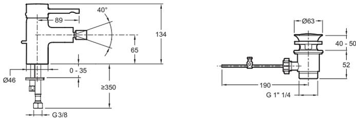
Product Specification: Single-lever bidet mixer. 37045D. Collection: CÜFF. Weight: 1.5 kg. Installation: 1 hole. Normes: ACS (Certificate of Sanitary Compliance): 10 ACC LY 102. Flow rate: 5 l/mn. Faucet drilling: 1 faucet hole. Flow rate: 5 l/mn. Height under spout: 134 mm. Connection: With supply hoses. Mechanism: Ceramic disc cartridge. Side lift rod. No base plate for easier cleaning. Waste. Rotating anti-scale aerator. Finger imprint on handle. Height under aerator: 65 mm. 5-year guarantee.
