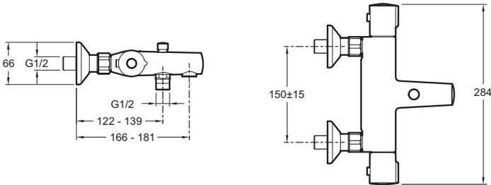
Product Specification: Thermostatic single-lever wall-mount bath/shower mixer. 45714D. Collection: JULY. Installation: Wall-mount. Flow rate: 21 l/min. Connection: With connectors and wall escutcheons. Safety stop at 37°C. maximum temperature 50°C. Non-return valve on supply connections. Connectors with wall escutcheons. Anti-scale aerator. Discreetly-positioned automatic diverter.
