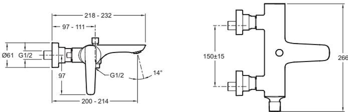
Product Specification: Single-lever wall-mount bath/shower mixer. 72319D. Collection: ALEO+. Installation: Wall-mount. Flow rate: 20 l/mn. Connection: With connectors and wall escutcheons. Non-return valve on shower outlet. Connectors with wall escutcheons. Ceramic disc cartridge. Automatic diverter.
