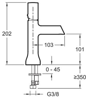
Product Specification: Tall single-lever washbasin mixer. 7329D. Collection: T00BI. Weight: 1.3 kg. Installation: 1 hole. Flow rate: 8 l/min. Flow rate: 8 l/min. Connection: With supply hoses. Mechanism: Ceramic disc cartridge. No drain. Ceramic disc cartridge. Green, white and black spout inserts.
