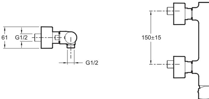
Product Specification: Single-lever wall-mount shower mixer. 8962D. Collection: TOOBI. Weight: 1.7 kg. Installation: Wall-mount. Flow rate: 15 l/min. Connection: With connectors and wall escutcheons. Mechanism: Ceramic disc cartridge. Hole configuration:  $150 \pm 15$  mm. Pop art inspiration.
