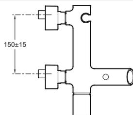
Product Specification: Single-lever wall-mount bath/shower mixer. 8963D. Collection: TOOBI. Weight: 2.6 kg. Installation: Wall-mount. Flow rate: 30 l/min. Flow rate: 30 l/min. Connection: With connectors and wall escutcheons. Mechanism: Ceramic disc cartridge. Hole configuration: 150 ± 15 mm. Pop art inspiration. Automatic diverter. Integrated handshower holder. 2 spout inserts (white and green) for personalization.
