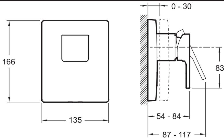
Product Specification: Trim and lever for built-in shower mixer. 98632D. Collection: MODULO. Weight: 2.1 kg. Installation: Wall-mount. Normes: ACS (Certificate of Sanitary Compliance): 10 ACC LY 004. Incl. single-lever built-in mixer. Incl. non-return valve. Ceramic disk cartridge. DVGW NW-6512CP0427.
