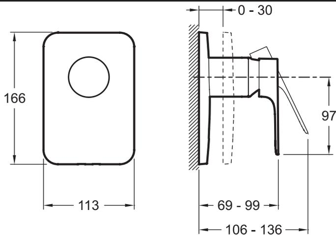
Product Specification: Trim and lever for built-in shower mixer. 98706D. Collection: ALEO+. Installation: Wall-mount. Mount with Modulo universal box 98699D-NF. Kit composed of built-in body, trim, handle and diverter. Easy-to-install cartridge, thanks to guide notches. Ceramic disk cartridge.
