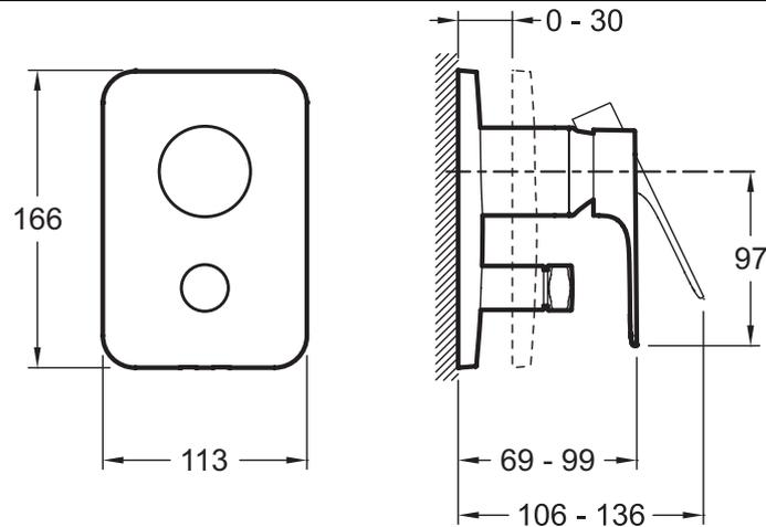
Product Specification: Trim and lever for built-in bath/shower mixer, 98718D. Collection: ALEO+. Installation: Wall-mount. Mount with Modulo universal box 98699D-NF. Kit composed of built-in body, trim, handle and diverter. Easy-to-install cartridge, thanks to guide notches. Automatic diverter with locking option. Non-return valve.
