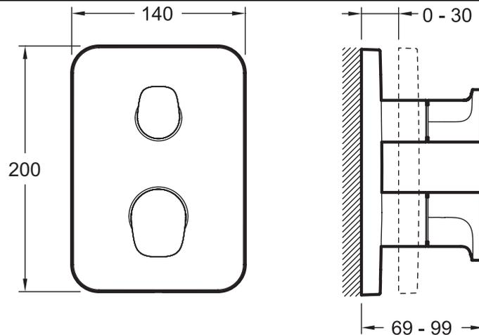
Product Specification: Hybrid trim for built-in bath/shower mixer. 98730D. Collection: MODULO. Installation: Wall-mount. Incl. thermostatic and flow-control valve. Instantaneous water heater suitable. Filter and non-return valves. DVGW NW-6512CP0430.
