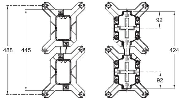
Product Specification: Box connector to align 2 superposed boxes. 98788D. Collection: MODULO. Installation: Built-in. Install to connect two Modulo universal boxes 98699D-NF. Easier alignment of two boxes. perfect esthetics. Better seal between the two boxes.
