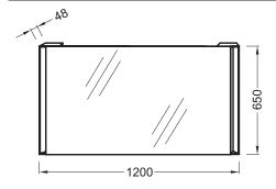
Product Specification: Mirror 120 cm. EB577. Collection: RÊVE. Dimensions: 120 x 5 x 65 cm. Weight: 14.8 kg. Installation: Wall-mount. Power: 230 V, 2 x 24 W, T4 fitting, class II, IP44, energy efficiency class A. Note: the infrared sensor switch requires a gap of at least 15 cm between itself and the tile or other object.
